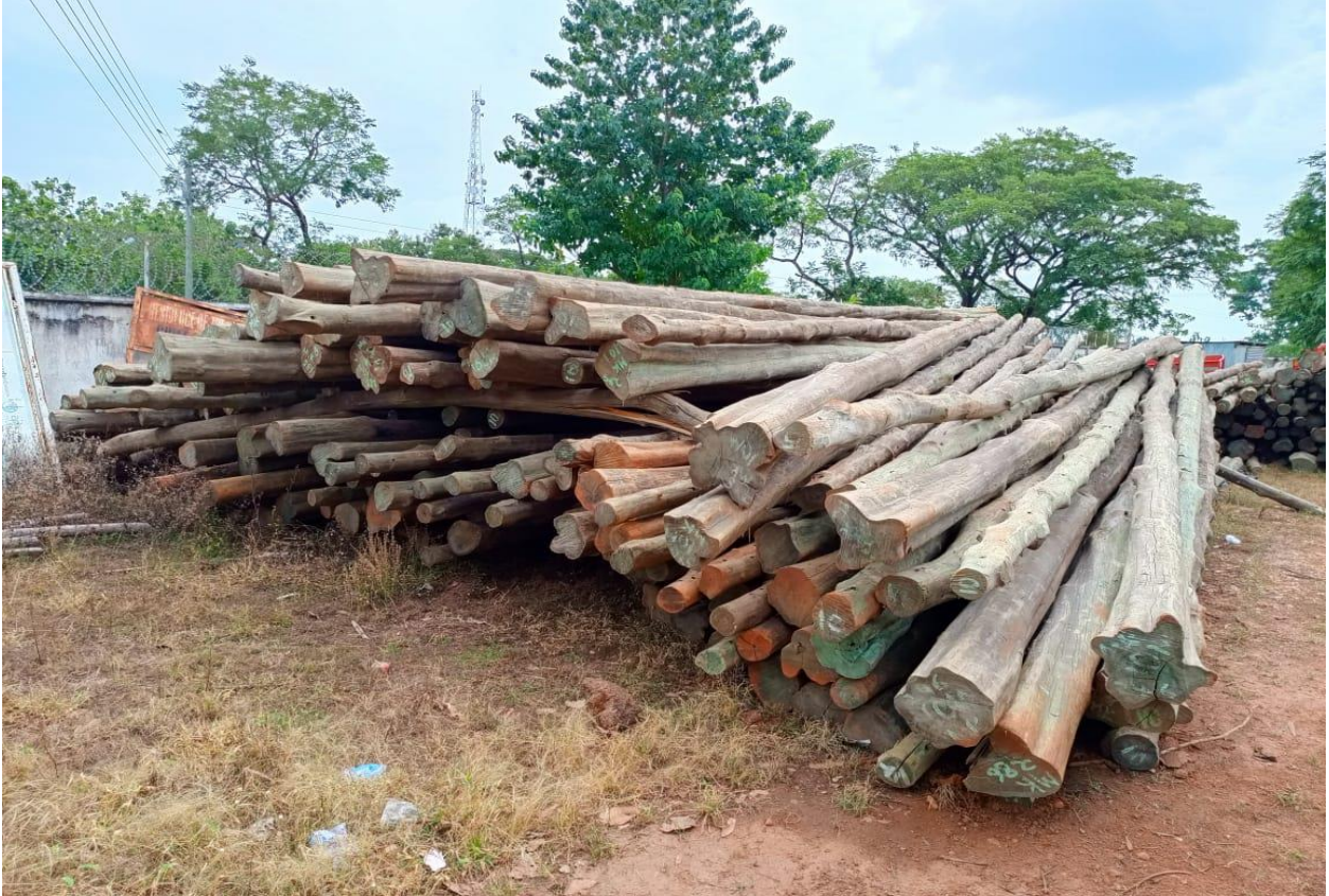
Supplied 90 Electricity Poles for distribution
